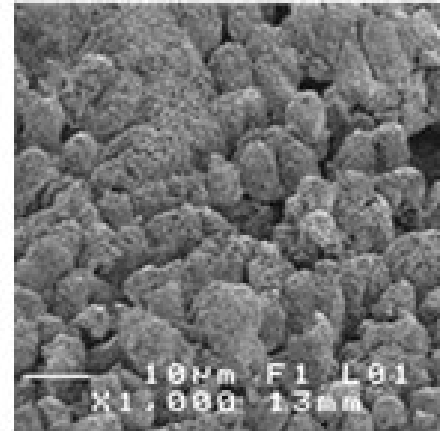
Left: SEM image of surface produced within the project. Right: SEM image of the surface of a Lotus leaf. (D. Chakarov, P. Holgerson)
